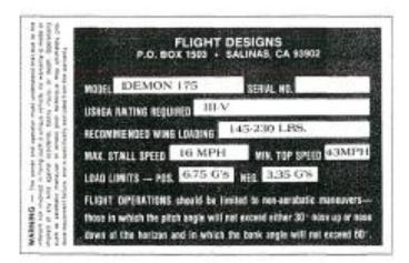
These placards are located on the keel, on the right hand side, near the control bar bracket.
